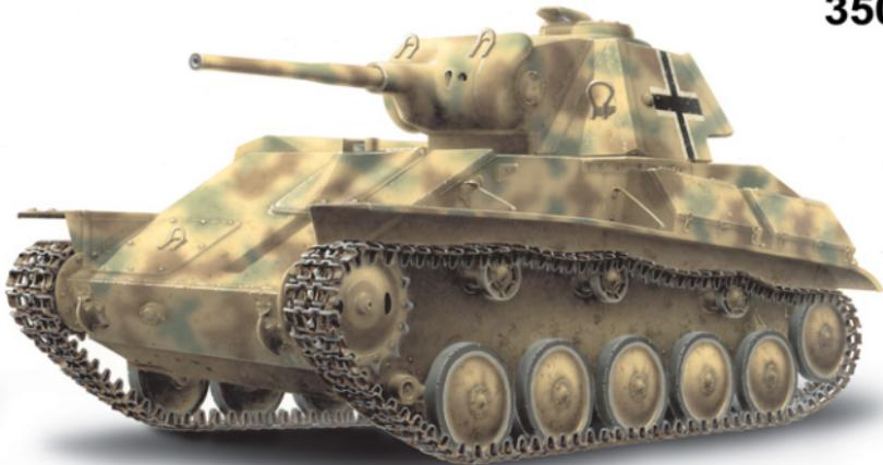
Light tank T-70 was designed in 1944 instead of light tank T-60. The mass production began since 1942. In September 1942 manufacture of updating T-70M began will increased moving part, the changed hach for mechanic-driver and other changes. Production ceased in autumn 1943. During this period 8226 Tanks T-70 and T-70 M more released at the Gorkij, Sverlovsk and Kirov military factory.
